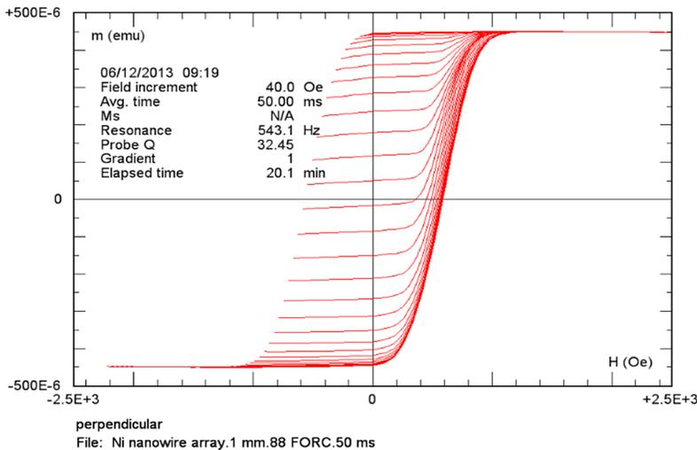
Figure 3: First-order-reversal-curves (FORC) for an array of Ni magnetic nanowires (sample courtesy of L. S. Spinu<sup>5</sup>.)
