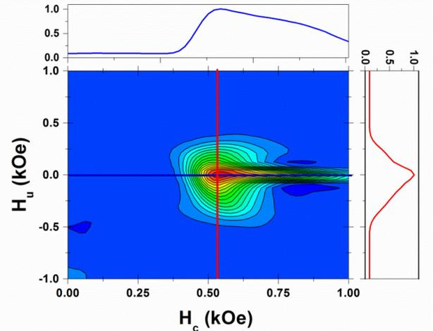
Figure 4: Distribution of interaction fields as determined from FORC analysis
