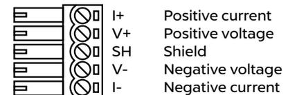
**NOTE:** Make sure to properly seat connectors. When removing a sensor, use a screwdriver to gently remove the connector.
