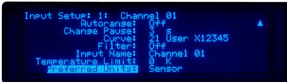
11. Press **Escape** to go back to the main screen, which will now display a temperature reading. You will notice that the resistance reading is still visible, displayed as Impedance on the right side of the screen. For more information, please see section 2.5.3 of the Model 372 user's manual.
