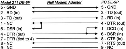
**NOTE:** Same as null modem cable design except PC CTS is provided from the Model 211 on DTR.
