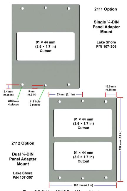
Figure 2-5. 2111 and 2112 Panel Mount Adapters
