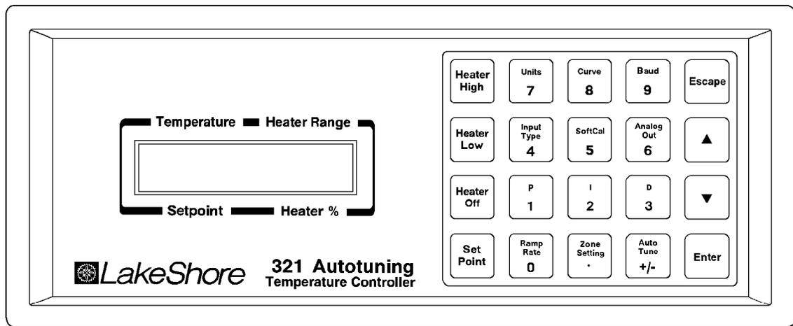
Figure 3-1. Model 321 Front Panel
