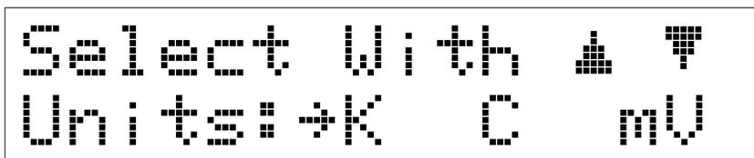
Use the ▲, ▼, or **Units** button to cycle the selector arrow (→) between choices. The available selections are K (kelvin), C (Celsius), and mV (millivolts). Display in K is the default value. Press **Enter** to accept the new units or **Escape** to return the normal display and retain the old setting.
