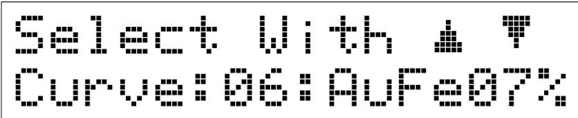
A rectangular box containing two lines of pixelated text. The first line reads "Select With" followed by an up arrow and a down arrow. The second line reads "Curve: 06: AuFe07%".
