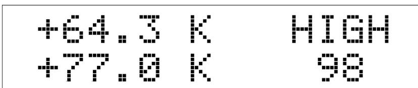
The percentage of current reflects the percentage of full scale current being applied to the heater output, and will change automatically according to control parameters.
