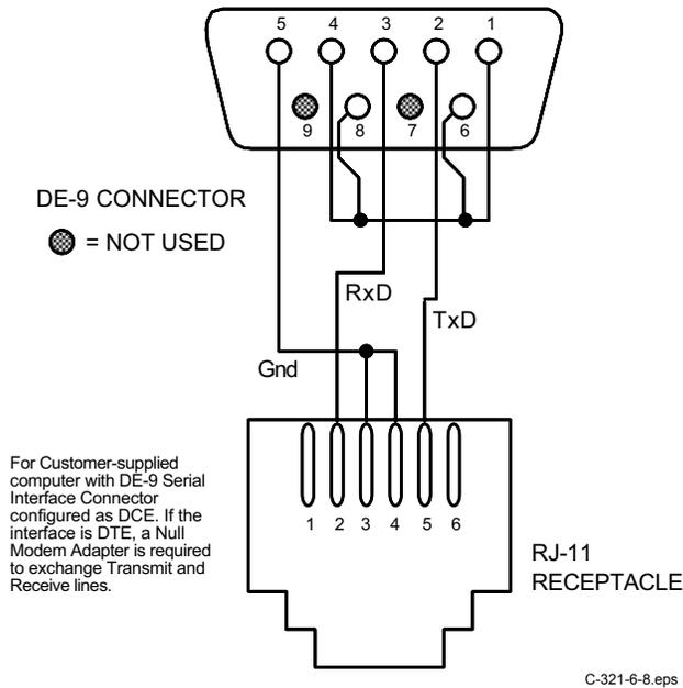
Figure 6-8. Model 2003 RJ-11 to DE-9 Adapter Wiring Details
