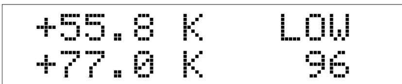
The heater high output is 25 Watts maximum into 25  $\Omega$ . A typical **Heater High** display is shown as follows.
