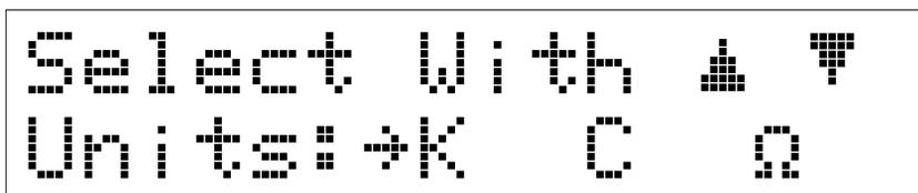
Use the ▲, ▼, or **Units** button to cycle the selector arrow (→) between choices. The available selections are K (kelvin), C (Celsius), and Ω (ohms). Display in K is the default value. Press **Enter** to accept the new units or **Escape** to return the normal display and retain the old setting.
