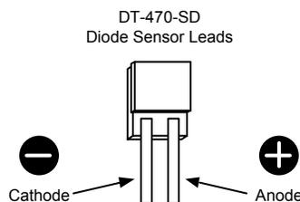
On the DT-470-SD, the base is the largest flat surface. It is sapphire with gold metallization over a nickel buffer layer. The base is electrically isolated from the sensing element and leads, and all thermal contact to the sensor should be made through the base. A thin braze joint around the sides of the SD package is electrically connected to the sensing element. Contact to the sides with any electrically conductive material must be avoided.
