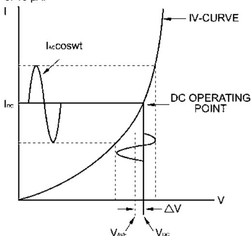
FIGURE 2. IV curve for a silicon diode sensor showing effect of an induced ac current superimposed on the dc operating current  $I_{dc}$ . The expected dc operating voltage is  $V_{dc}$ , which is shifted from the average voltage  $V_{ave}$  indicated by the voltmeter in a dc measurement mode.
