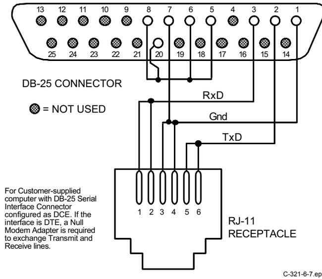
Figure 6-7. Model 2002 RJ-11 to DB-25 Adapter Wiring Details
