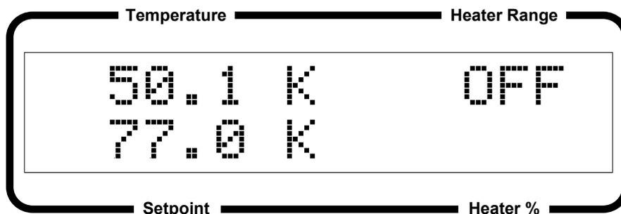
When the heater is on, **Heater %** will reflect the percentage of current being applied to the heater. The heater low output is 2.5 Watts maximum into 25  $\Omega$ . A typical **Heater Low** display is shown as follows.
