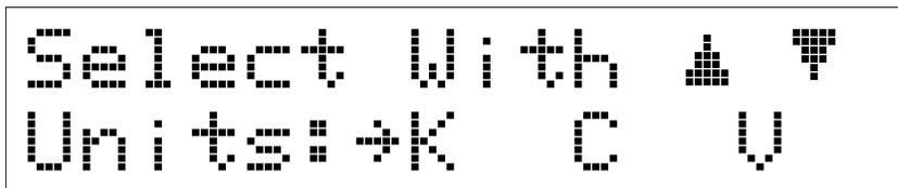
Use the ▲, ▼, or **Units** button to cycle the selector arrow (→) between choices. The available selections are K (kelvin), C (Celsius), and V (Volts). Display in K is the default value. Press **Enter** to accept the new units or **Escape** to return the normal display and retain the old setting.
