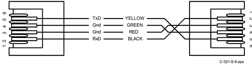
Figure 6-6. Model 2001 RJ-11 Cable Assembly Wiring Details
