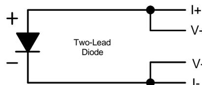
The error in a resistive measurement is the resistance of the lead wire run with current and voltage together. If the leads contribute 2 or 3  $\Omega$  to a 10 k $\Omega$  reading, the error can
