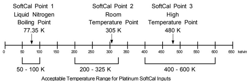
**Figure 8-2. SoftCal Temperature Ranges for Platinum Sensors**
