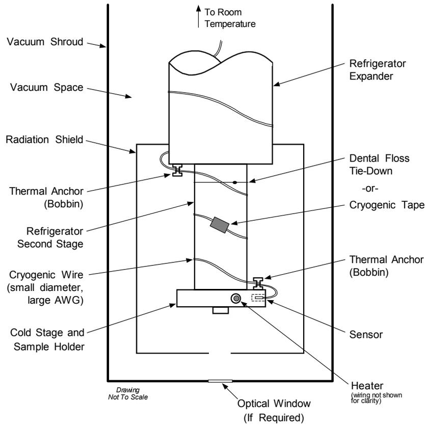
Figure 2-2. Typical Sensor Installation In A Mechanical Refrigerator
