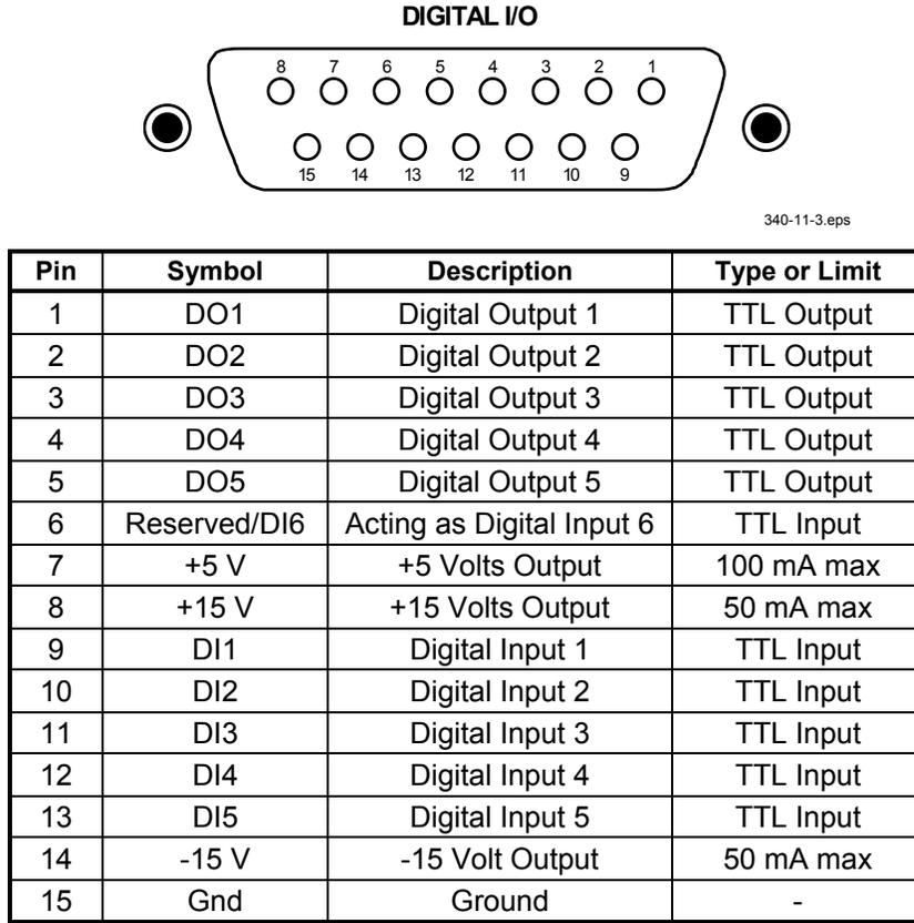
**Figure 11-4. DIGITAL I/O DA-15 Rear Panel Connector Details**
