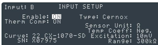
The user can select the sensor type and the controller will automatically select the sensor units, excitation and range. If "special" type is selected, the user can choose any available excitation and input range.
