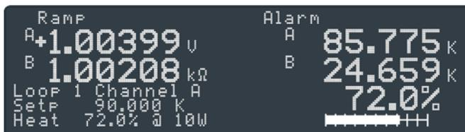
This shows a variation of the display with a large loop 1 heater output graphic bar where the PID parameters are not displayed, but the heater output is more prominent.
