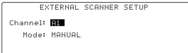
The digital outputs must be set to scan mode to report the scan channel. Refer to Paragraph 7.2 for digital output mode setting. When the digital outputs are set to work with the scanner and manual scan mode selected, digital output signals D1 to D4 report the active scan channel as shown below. Digital output logic levels are described in Paragraph 7.2.
