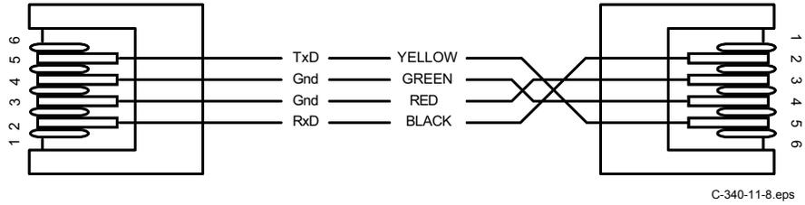
Figure 11-10. Model 2001 RJ-11 Cable Assembly Wiring Details
