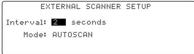
The digital outputs must be set to scan mode to report the scan channel, refer to Paragraph 7.2 for digital output mode setting. When the digital outputs are set to work with the scanner and Auto Scan mode selected, digital output signals D1 to D4 report the active scan channel as shown in the table above.
