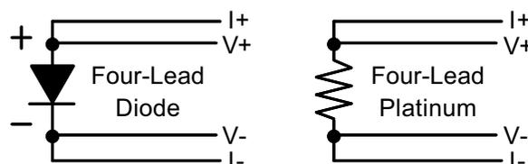
In a four lead measurement, current leads and voltage leads are run separately up to the sensor. With separate leads there is little current in the voltage leads so their resistance does not enter into the measurement. Resistance in the current leads will not change the current as long as the voltage compliance of the current source is not reached. When two lead sensors are used in four lead measurements, the short leads on the sensor have an insignificant resistance.
