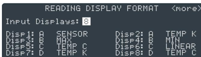
The user can display 1 to 8 readings from any of the available inputs. The units available are the sensor units of mV, V,  $\Omega$ , k $\Omega$ , nF or temperature units of  $^{\circ}\text{C}$  or K. Results of the math feature can also be selected.
