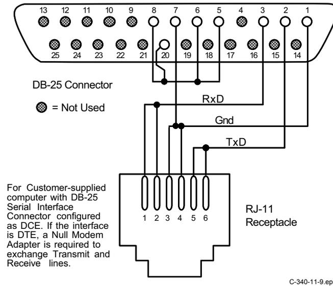
Figure 11-11. Model 2002 RJ-11 to DB-25 Adapter Wiring Details
