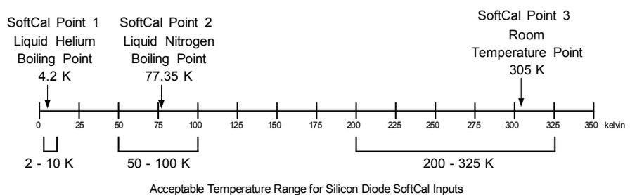
**Figure 8-1. SoftCal Temperature Ranges for Silicon Diode Sensors**
