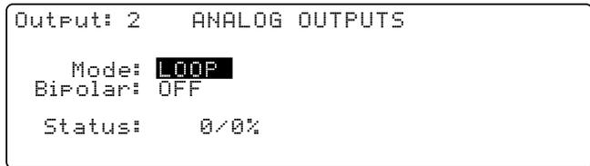
It is recommended to set the Analog Output to unipolar mode. Few applications can use bipolar control output. A thermoelectric cooling element is one example of a control actuator that can utilize a bipolar control output. The AutoTune feature will not operate with Loop 2 configured for Bipolar Control.
