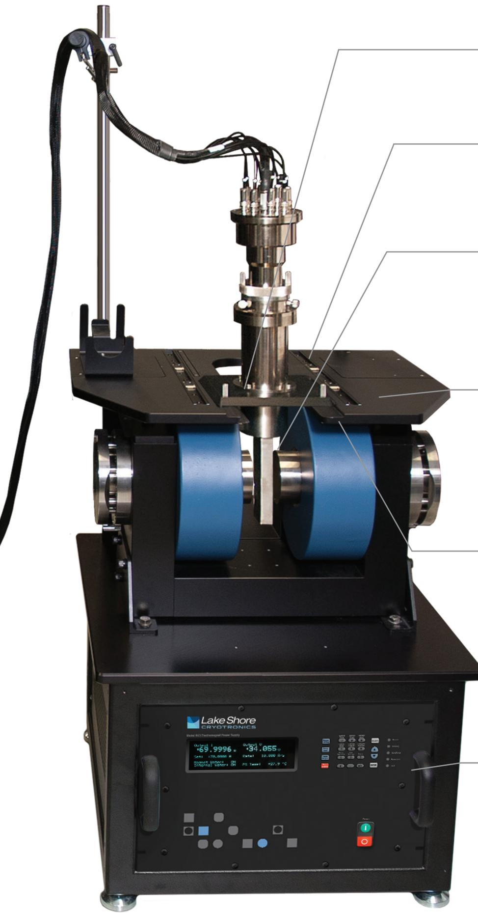
**Easy setup** — for ease of sample module exchange, modules slide forward out of the magnet gap
