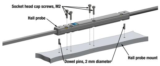
Figure 4. Exploded view of suggested mounting hardware
