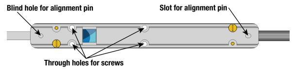
Figure 2. Mounting provisions on the mountable Hall probe handle
