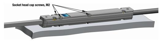
Figure 5. Probe handle mounted with suggested hardware
