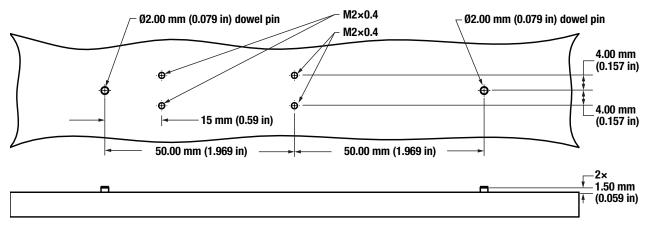
Figure 3. Mountable probe suggested mounting interface
