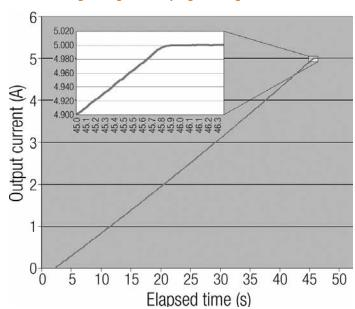
This plot illustrates an actual 5 A current change into an  $8.6~\mathrm{H}$  superconducting magnet. A smooth, 95 mA/s ramp is shown with minimal overshoot highlighted in the detail area. (Output current monitor measured at  $58.88~\mathrm{Hz}$  rate with a HP  $34401-\mathrm{data}$  multiplied by  $10\times$  to obtain output current results.)
