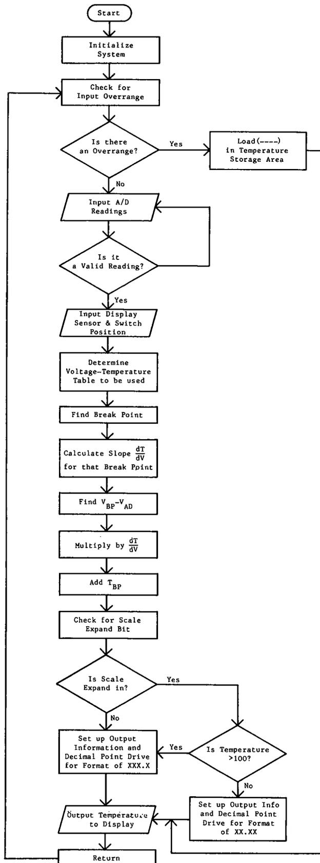
FIGURE 4.1 Software Flow Diagram for DRC-80 Digital Thermometer
