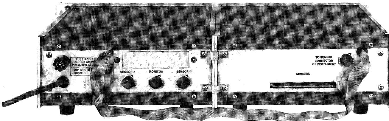
FIGURE 3.5 Model DRC-80 and SW-10A Rear View showing RM-3H Rack Mounting Hardware and Umbilical Cord Connections.
