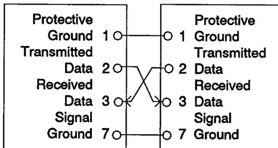
**NOTE** It may be necessary to jumper pins 5, 6, 8 and 20 to disable the handshake functions of the Host. This is not required for the 8223 Interface.
