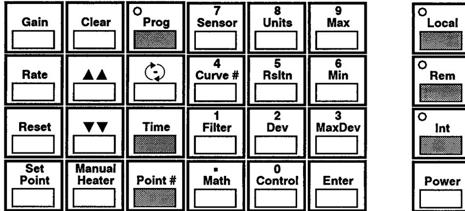
The Program (*Prog*) key, the Internal (*Int*) key and the Time key are used when utilizing the Internal Programming feature. Please reference the Internal Programming discussion of this section for description of this feature.
