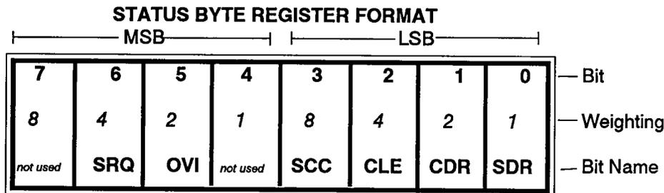
If the Service Request is enabled, any of the bits (0-5) being set will cause the unit to pull the SRQ management line low to signal the BUS CONTROLLER. These bits are reset to zero upon a serial poll of the Status Byte Register. These reports can be inhibited by turning their corresponding bits in the Service Request Enable Register to off.
