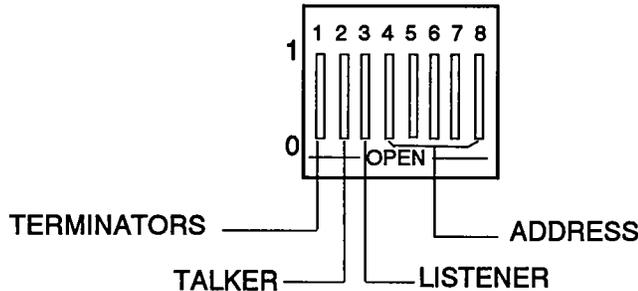
For the default of 12, address switch numbers 5 and 6 will be CLOSED (1) which will result in the Address Switch having a setting of 00001100 or 10001100 dependent on the requirements for the terminators.
