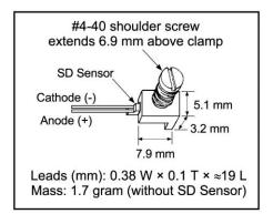
sides of the SD sensor and is electrically connected to the sensing element. Contact to the sides with any electrically conductive material will cause a short.
