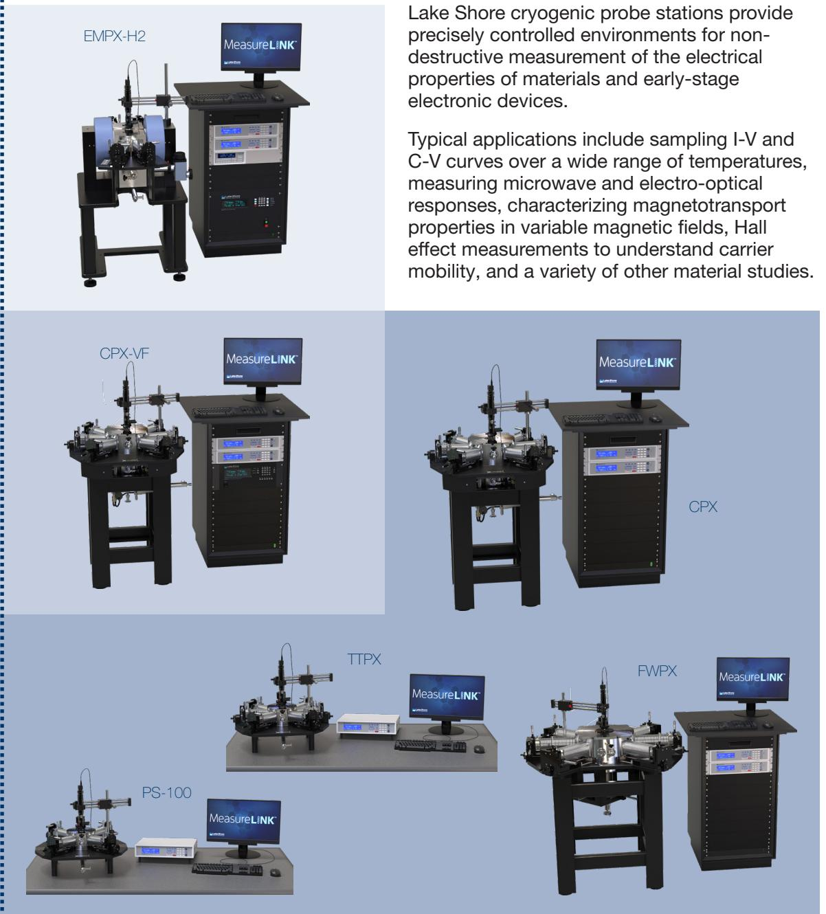
Lake Shore cryogenic probe stations provide precisely controlled environments for non-destructive measurement of the electrical properties of materials and early-stage electronic devices.
