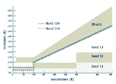
**DT-400 Series Expanded Temperature Response Data Table**
